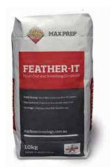
**Universal** | Suitable for most floor coverings **Easy to install** | 2.5mm to 20mm in one application **Mixing ratio** | 4.5 litres of water to 20kg powder **Coverage** | 20kg bag covers 4m<sup>2</sup> at 3mm thickness
