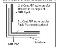
Tiling can begin once the second coat has dried which is generally 3 hours at 23 °C in undertile applications. Drying times will vary depending on humidity, surface temperature and porosity of substrates. The membrane must be lapped to penetrations such as waste outlets in accordance with AS 3740.
