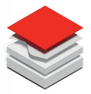
**FULLY ADHERED SYSTEM** Membrane panels are fully adhered directly to an acceptable substrate
