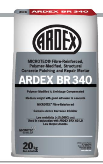
ARDEX BR 340 Structural Concrete Patching and Repair Mortar is designed for reinstating concrete surfaces damaged through concrete spalling and other chemical or mechanical causes. ARDEX BR 340 is a high-build patching mortar and is capable of being applied up to a thickness of 80mm on vertical, horizontal and overhead surfaces.
