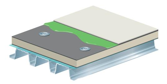
The UltraPly™ TPO fully adhered system is a lightweight system with outstanding design flexibility. It is suitable for roofs that are designed with a need for aesthetics, roofs with irregular shape, contoured roofs and any roof with limited load bearing capacity, provided the substrate is compatible with adhesive. It is the preferred system for green roofs, parking decks and roofs with photovoltaic installations.
