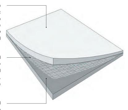
Firestone's UltraPly TPO roofing membrane is constructed in a way that at least 40% of the top ply weathering layer is above the scrim layer (at the scrim location), which provides outstanding weather resistance to the membrane.
