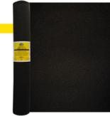
ARDEX DS 70 is a high-performance, resilient rubber flooring underlayment for the reduction of impact sound, decoupling and crack isolation under hard floorcoverings. ARDEX DS 70 is made from 92% post-consumer recycled, wear and water resistant rubber granules and is rated to provide a 14dB improvement. ARDEX DS 70 also acts as a decoupling mat to isolate cracking and substrate movement from the flooring finish.
