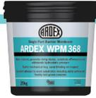
ARDEX WPM 368 is a single component acrylic co-polymer membrane that will prevent rising damp, efflorescence and will resist negative hydrostatic pressure when used in accordance with the technical data sheet. It has excellent adhesion to most substrates including brick, masonry, concrete block, concrete and stone and is simple to use by brush, roller or airless spray machine.
