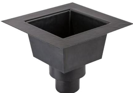
Moulded rainhead, 295mm square. To suit 100mm or 150mm downpipe. 50mm rim allows for 50mm seam tape on edge.
