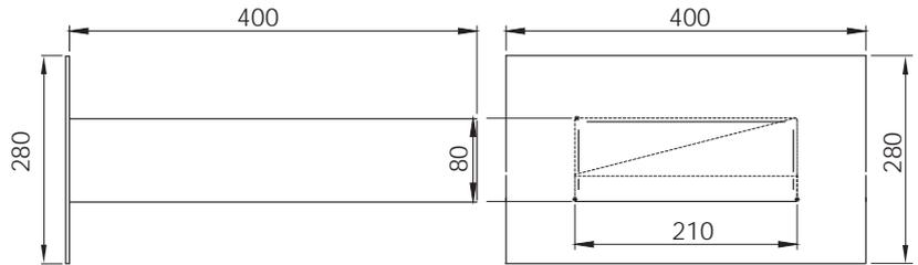
Allows overflow to take rainwater safely through parapet wall. 210mm channel with a 2° fall.
