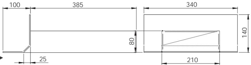
Allows overflow to take rainwater safely through parapet wall. 210mm channel with a 2° fall. Meets E2/AS1 requirements.
