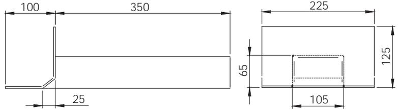
Allows overflow to take rainwater safely through parapet wall. 105mm channel with a 2° fall.
