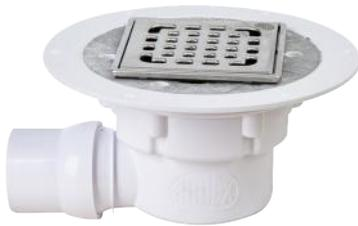
Side exit clamp waste unit with removable soap strainer. Welds to the outside of DWV50.
