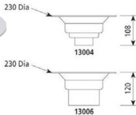
Bottom exit clamp waste unit with removable soap strainer. Welds to the outside of DWV50 / DWV80 and DWV100.
