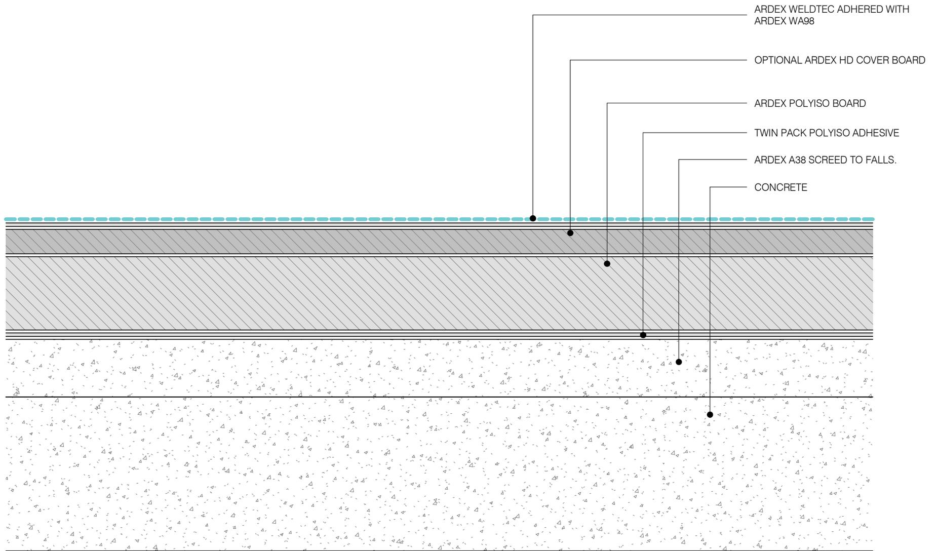
NOTE: FOR FASTENING OR FIXING PATTERN DEPENDENT ON WIND ZONE/R VALUES.
