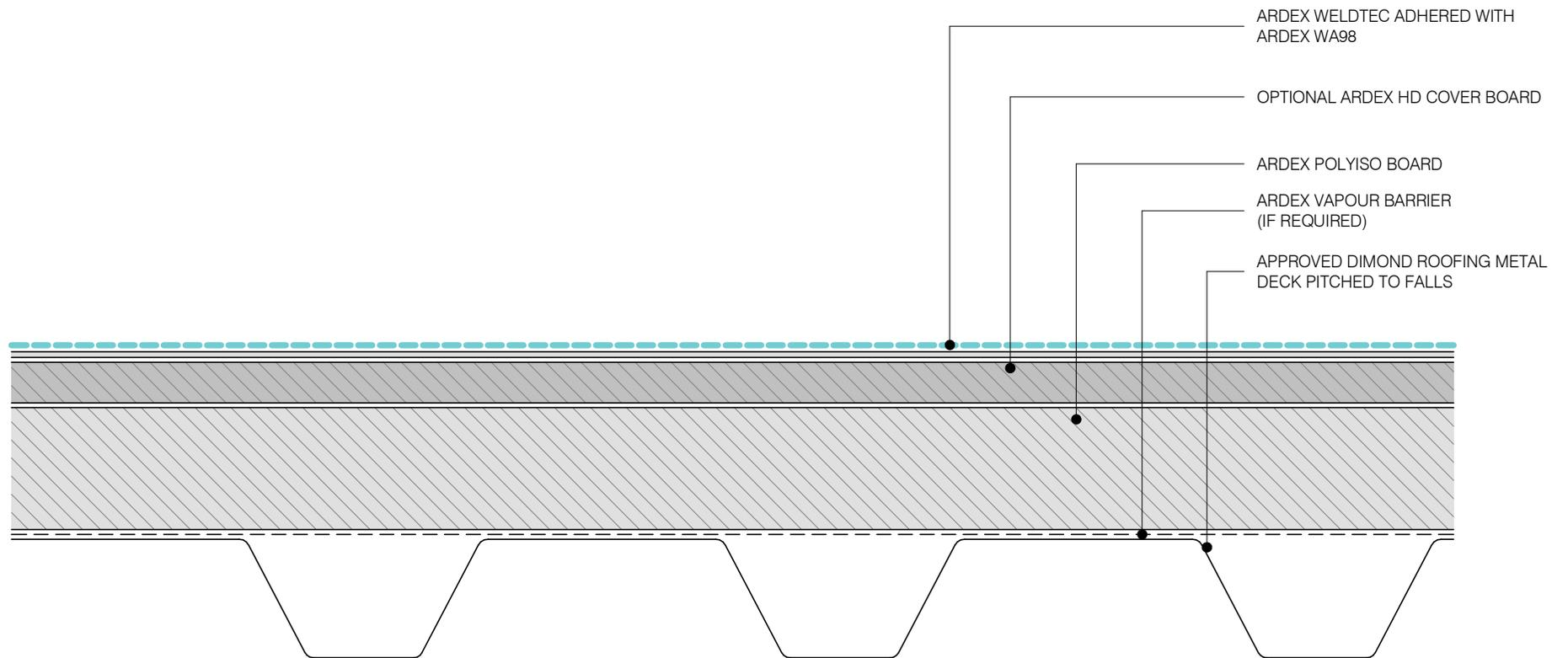
NOTE: FOR FASTENING OR FIXING PATTERN DEPENDENT ON WIND ZONE/R VALUES.
