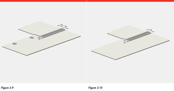
Firestone recommends for welds made with an automatic welder a minimum width of 38 mm and for welds made with hand welders a minimum width of 50 mm.
