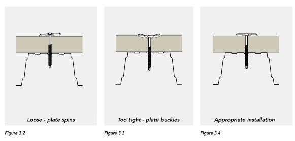
Under-driving the fasteners will result in a loose plate with insufficient clamping force and a protruding fastener head. Both situations could cause damage to the membrane during normal foot traffic.
