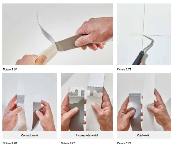
All welds systematically require a combination of visual inspection, mechanical testing and destructive testing to assure a consistent quality of the welded seams.
