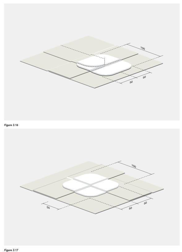
For single T-joints a standard cut T-joint cover piece of 100 x 100 mm should be installed.
