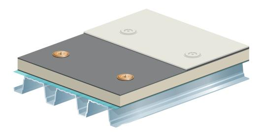
The UltraPly™ TPO induction welding system is a variation of the conventional mechanically fastened system. It is commonly used on buildings where the deck is suitable for mechanical attachment and where the application of a mechanically attached system is not practical due to high wind uplift requirements.
