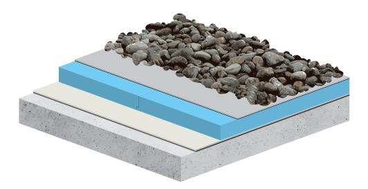
The UltraPly™ TPO inverted system is a variation of the conventional ballasted system. It is suitable for projects with regular traffic and for roofs that are vulnerable for internal condensation.
