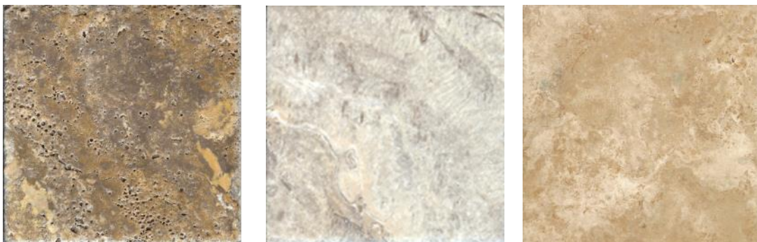
Travertine limestone tiles—These tiles often show marking which starts at the voids in the rock structure. They can be filled with grout to fill the voids.
