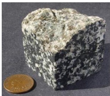
An example of Granodiorite. These are commonly more melanocratic than true Granite, and contain Plagioclase as the main Feldspar.
