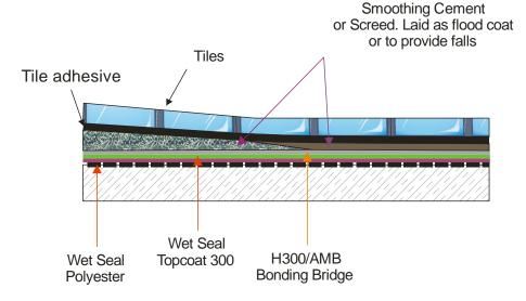
Example of a non-heated subfloor with smoothing cements and created falls.
