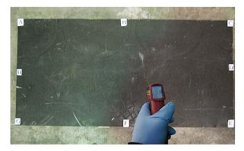
Conducting a sun exposure trial of a large format 'blue stone tile'. Measuring the surface temperature of the tile. The letters mark the positions for measurement with a straight edge laid across the tile. This measures the unrestrained movement of the tile.
