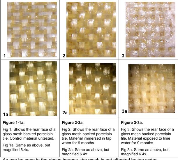
As can be seen in the above images, the mesh is not affected by tap water, however lime water produced breakdown of the glass mesh, which could be scraped away.
