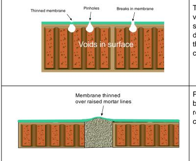
This is a situation where voids in the underlying surface can lead to development of pinholes or thinning of the membrane / coating.
