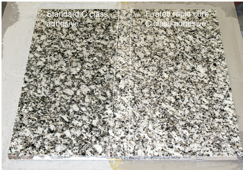
Figure 11. An unusual porphyritic granite (Adamellite) displaying extreme sensitivity to marking. The left side of the tile was bonded with a C2TES1 adhesive and on the right a C1FT adhesive intended for sensitive tiles. The central strip shows the natural colour. As can be seen, shade change occurred even with the F rated fast cure adhesive. This tile requires 100% adhesive coverage to display a consistent colouring.
