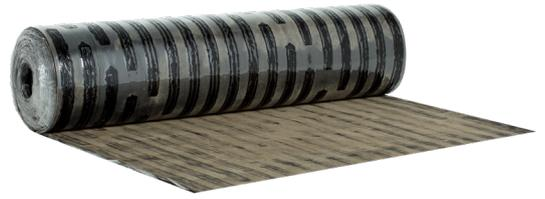
ARDEX WPM 114 is an APP (Atactic Polypropylene) plastomeric-type, modified bitumen membrane vented base sheet consisting of a specially formulated bituminous compound of distilled asphalt modified with selected high-grade viscoelastic polymers. ARDEX WPM 114 is used as part of a multi-layer waterproofing system where there may be potential moisture issues in the substrate.
